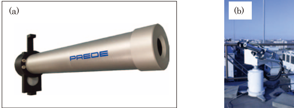
Fig. 1.2.6.4.2.-1. Solid view angle calibration tube (a) and a calibration tube mounted on a skyradiometer (b).
