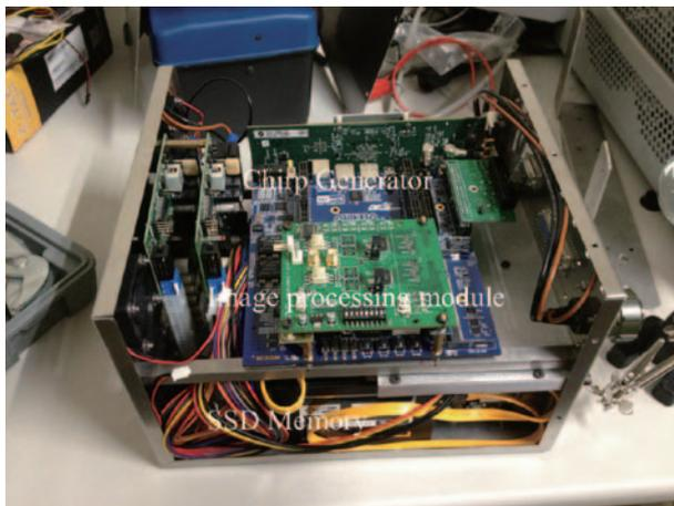
Fig. 1.1.1.-7. Chirp Pulse Generator and Image Processing module
