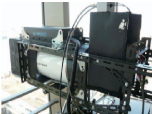
Fig.1 Compact lidar for horizontal atmosphere observation.
