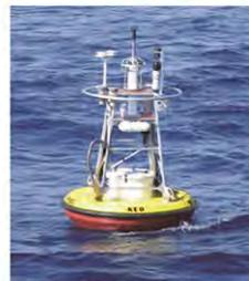
Fig.12 KEO buoy (Measurement height 4m, <http://www.pmel.noaa.gov/keo/>)
