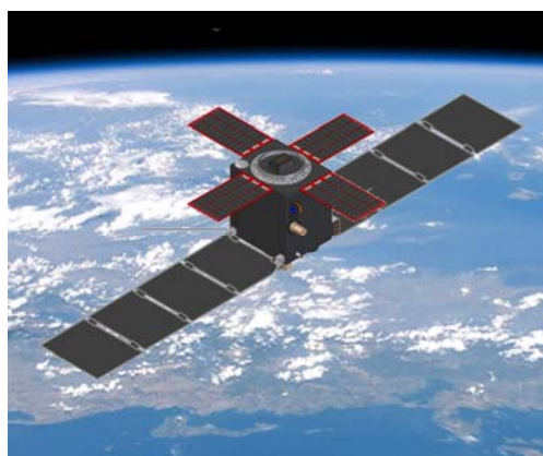
Fig.7. Illustration of CP-SAR onboard microsatellite
