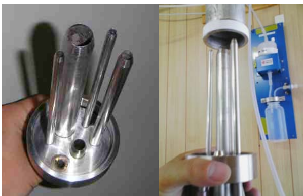
Fig. 3 Iso-kinetic air splitter of SKYNET community aerosol inlet.
