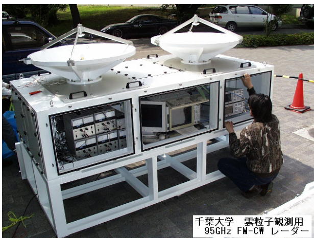
Fig.1. The developed cloud profiling FM-CW radar at 95 GHz.
