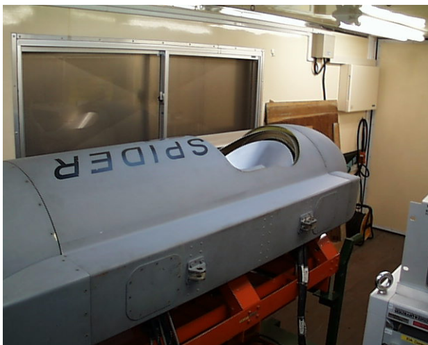
Fig.5. SPIDER: a pulse radar of the National Institute of Information and Communications Technology (NICT) Japan.
