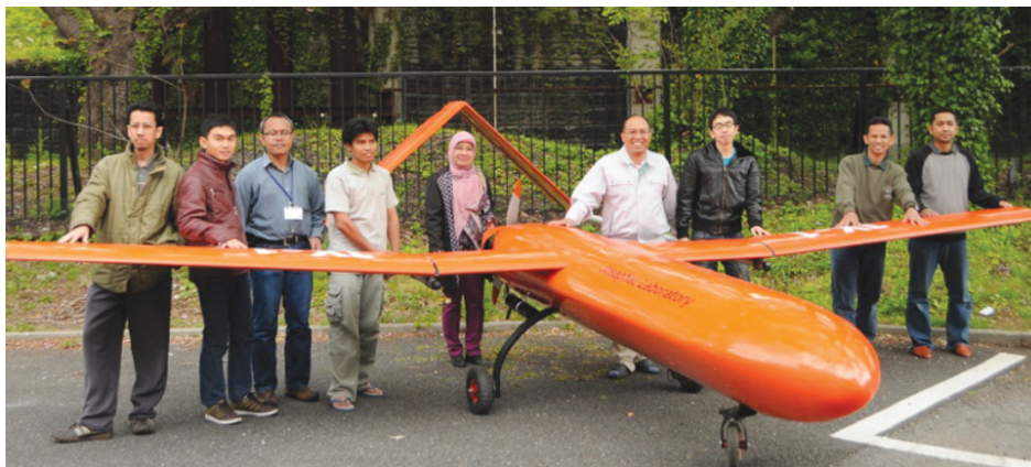
Figure 3. CP-SAR, GPS-SAR, and GPS-RO sensors onboard Josaphat Laboratory Experimental Unmanned Aerial Vehicle (JX-1).
