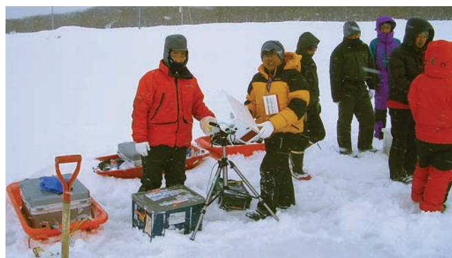
Figure 2. Prof Josaphat (yellow jacket) with students held ground survey to investigate the circular polarization of microwave characteristics of snow and ice at Saroma Lake, Hokkaido, Japan by using synthetic aperture radar (SAR) and microwave radiometer 18 GHz and 36 GHz.
