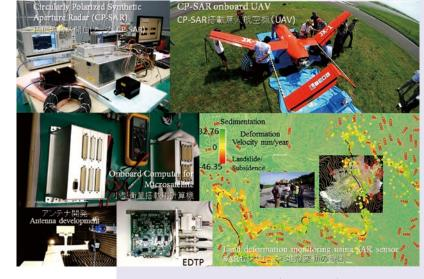
environment. The original sensor is circularly polarized synthetic aperture radar (CP-SAR) to monitor global land deformation, electron density – temperature probe (EDTP). In application development, CEReS develops differential interferometric SAR (DIn-SAR), permanent scatters interferometric SAR (PS-InSAR) etc to monitor land deformation and subsidence in several countries.
